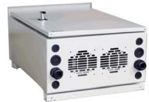
Wall-Mount Outdoor Fiber made of sheet EG Steel or stainless steel or Aluminium make to order one by one They can compliant with IP55 or IP 65 standard. they can accommodate the fiber from 12-96 Fiber support ST/SC/FC Cable entry 8 port use cable glands EG/PG29 depend on cable dia: 2 pcs. The cable can be held the preformed holes and LC, inside a 2 section cable inlet or cable feed through grommet. Application for CCTV or IP Camera.
